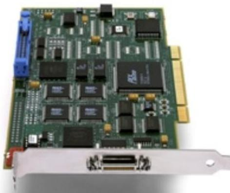
Figure 5.9 The R3-CL frame grabber board.
